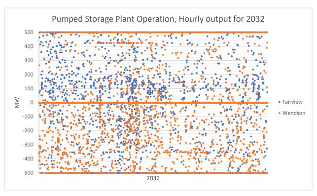
7 Figure 3: Raw output for the Rye Development pumped storage units
