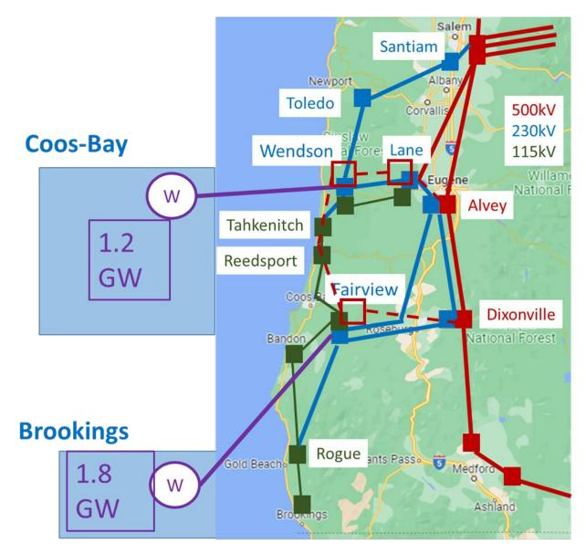
2 Figure 1: 2022 Offshore Wind Request with "500 kV loop"
