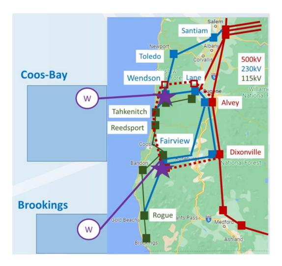
The 3 GW of offshore wind, 1.2 GW at Wendson and 1.8 GW at Fairview as well as the "500 kV loop" are modeled into the base cases used for this ESR analysis. The pumped storage project will be modeled as two, 500 MW pumped storage projects, each connecting at the 500 kV level at the Wendson and the Fairview buses.
